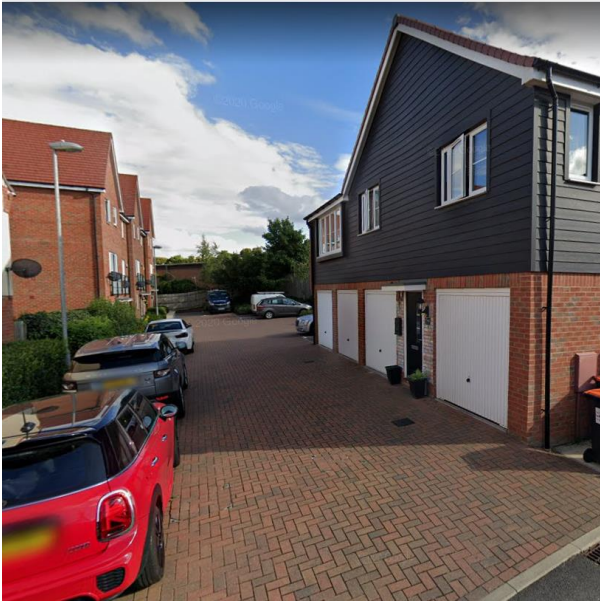
Vehicles parked opposite garages instead of inside them. Not enough space remains for a vehicle to get in or out of the garages.
