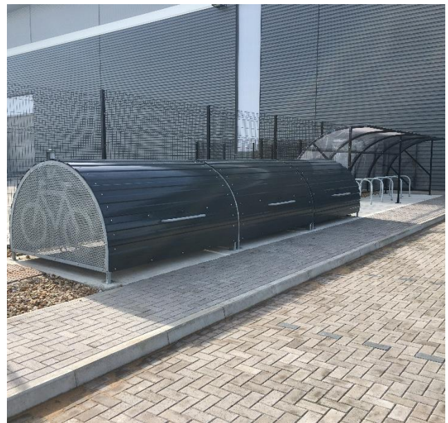
Lockable cycle hangars for long stay cycle parking and a shelter with Sheffield stands for short-stay cycle parking at an industrial unit.
