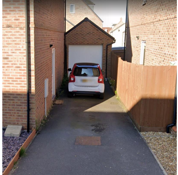
A driveway with boundary wall / fence both sides. Note how it would be difficult to use the side door to the house if another car was parked in the second parking space.
