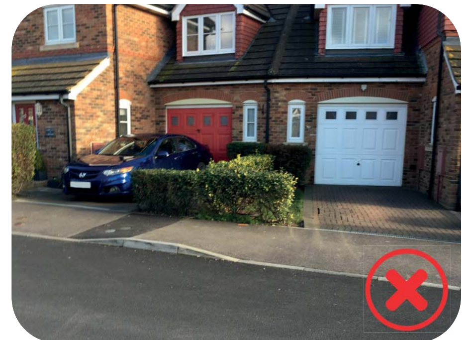
Short Driveway Leading to Overhang and Limited Garage Access, Thistle Hill, Minster
