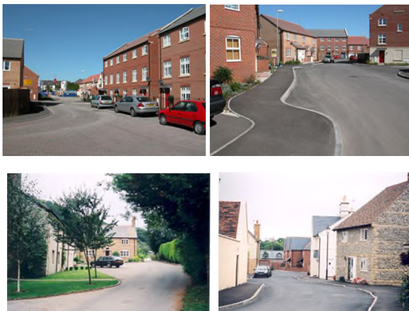
Figure DG18a Suggested on-street parking bays, parallel and perpendicular parking (top) and widening of carriageway to create on-street spaces (bottom). This Figure is based upon Figures 8.18 and 8.19 and paragraph 8.3.5.1 of the Manual for Streets documents. The Manual for Streets is copyright of the Department for Transport and Department of Communities and Local Government
