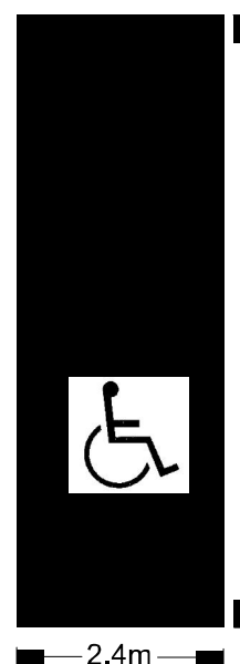
Bays in line
