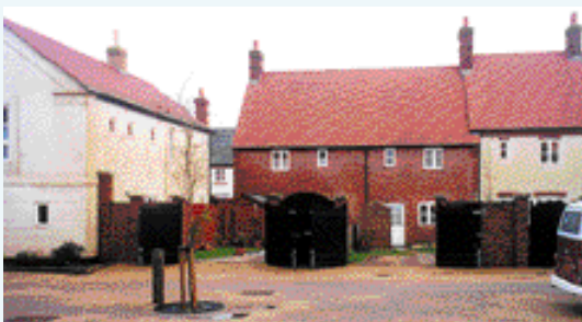
❺ While the amount of parking at Poundbury, Dorchester is high, its arrangement provides residents with the choice of in-curtilage parking or larger back gardens.
