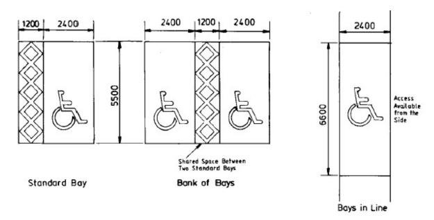
Off-street parking bays that are parallel to the access aisle, making access available from the side, should be at least 6.6m long and 2.4m wide. The additional length will allow access to the rear of the vehicle where wheelchairs are often stored. Access from the side should be unencumbered by street furniture.
