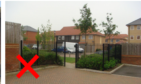
Rear parking courts must be secure and not "leaky"
