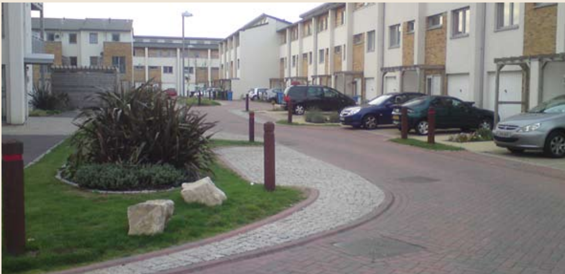
Over-run strip at junction
